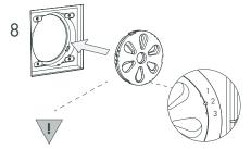
Check and Clean the Air Ventil regularly or replace with: PJ-AERO-R-FELT AIR VENTIL
