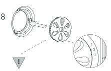
Check and Clean the Air Ventil regularly or replace with: PJ-AERO-R-FELT AIR VENTIL
