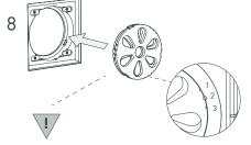
Check and Clean the Air Ventil regularly or replace with: PJ-AERO-R-FELT AIR VENTIL
